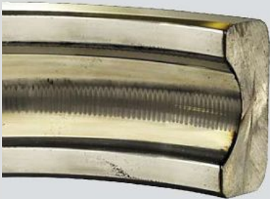
Bearing fluting, "washboard" pattern on bearing race
