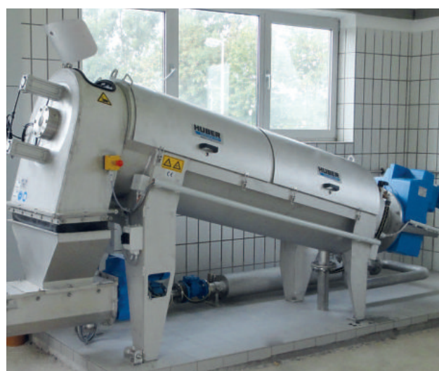
Stationary mounted screw press for 140 kgDS/h
