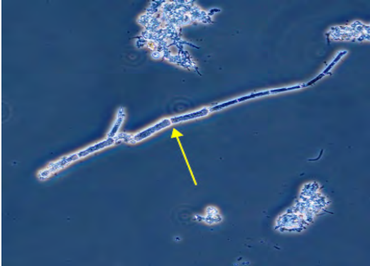
Figure 10 – Mixed Liquor 200X Phase Contrast Micrograph of Fungus Filament
