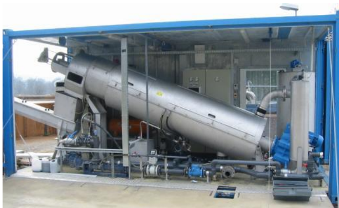
Containerized S-Press Design with Integrated Cake Conveyor
