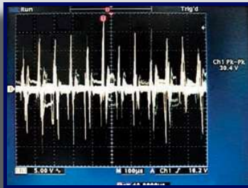
Shaft voltage reading with no protection
